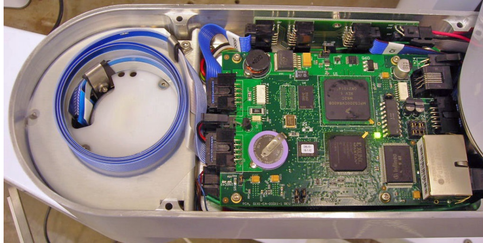
Controller Installed in Inner Link
