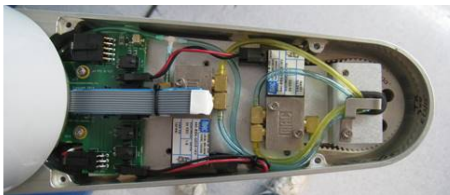
29. After installing the appropriate gripper, check Digital Input 1 for Pneumatic Gripper open sensor, Digital Input 2 for Pneumatic Gripper close sensor, and Digital Input 4 for vacuum present sense,
