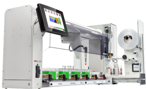
Easy access to load new capping foil
